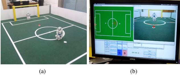
Fig. 3. Experimental setup - adversarial soccer penalty shooting task. (a): Initial poses of the autonomous striker (near side, blue waistband) and the teleoperated goalkeeper (far side, pink waistband). (b): Restricted perceptual information. Left: Visualisation of the robots’ self-localisation estimate (shown by the red markings on the field drawing). Right: Perspective view of the goalkeeper, looking at the ball and the approaching striker.
