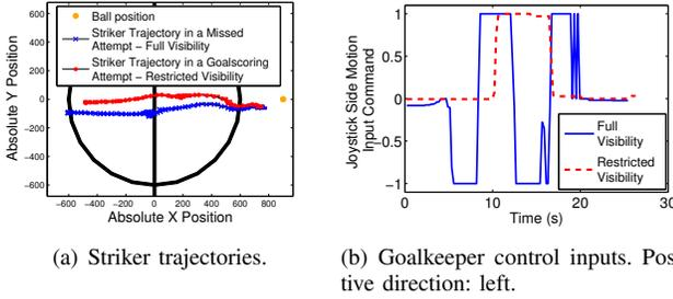
Fig. 12. Effects of idle time on performance of a specific subject. (a): Two similar trajectories by the striker against this subject, one per visibility case. Only the full visibility attempt was saved by the teleoperated goalkeeper. (b): Illustration of the variation of the subject’s side motion between these trials.
