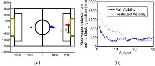
Fig. 8. Alternative performance metric for adversarial task: distance from optimal blocking position. (a): Explanation of metric. Poses of striker and goalkeeper at time of kick - optimal position for goalkeeper is the intersection of the line formed by the striker's orientation, and the goalkeeper's line of motion. (b): Results per subject, sorted by difference between visibility cases.
