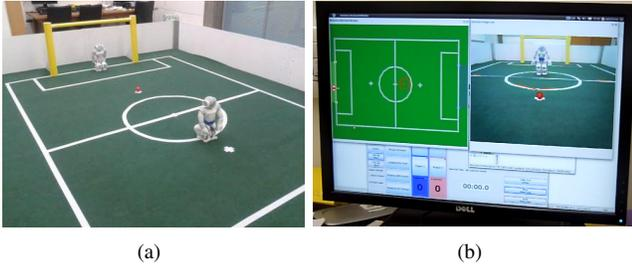
Fig. 3. Experimental setup - adversarial soccer penalty shooting task. (a): Initial poses of the autonomous striker (near side, blue waistband) and the teleoperated goalkeeper (far side, pink waistband). (b): Restricted perceptual information. Left: Visualisation of the robots’ self-localisation estimate (shown by the red markings on the field drawing). Right: Perspective view of the goalkeeper, looking at the ball and the approaching striker.
