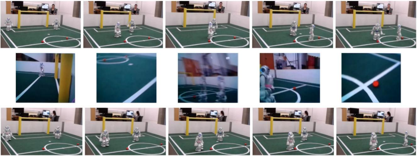
Fig. 4. Cooperative task. Navigation targets are now represented as orange balls. *Top*: A subject controlling the robot (blue waistband, starting at the right) under full visibility. *Middle*: A trial as seen through the teleoperated robot’s camera. *Bottom*: The same subject controlling the robot under restricted visibility.
