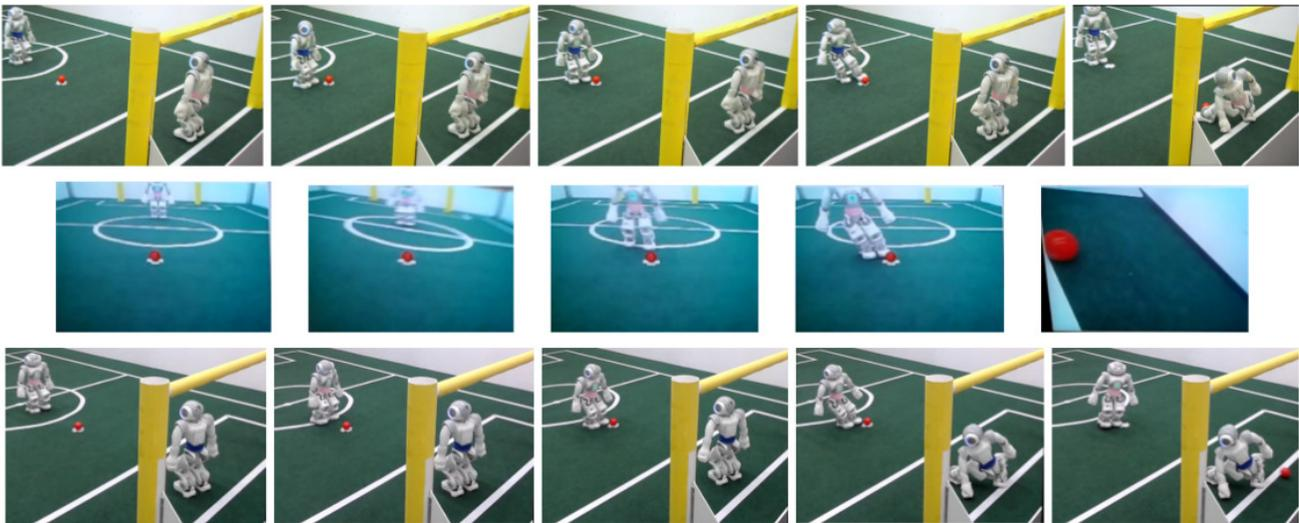
Fig. 5. Adversarial task. *Top*: Full visibility - a teleoperated goalkeeper (operator not shown) saves a shot. *Middle*: A trial as seen through the robot’s camera. The last snapshot shows the view of the goalkeeper after an unsuccessful dive to save the ball. *Bottom*: Limited visibility - different subject conceding a goal.
