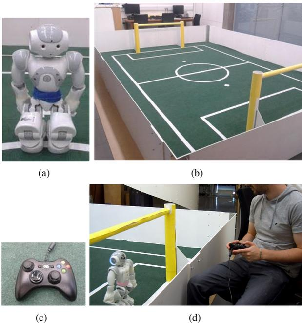
Fig. 1. Experimental setup. (a): The NAO humanoid robot. (b): The arena where the two robots interact. (c): The controller used to command the robot. (d): Remote control of a robot by a subject.
