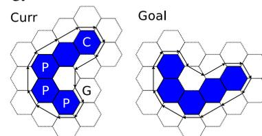
Fig. 4. Example of an error situation. Moving the unit at the only *CONTRACT* location to the only *GROW* location (thus forming the configuration in Figure 2) causes a kink violation *i.e.* the *StoS* planner is stuck
