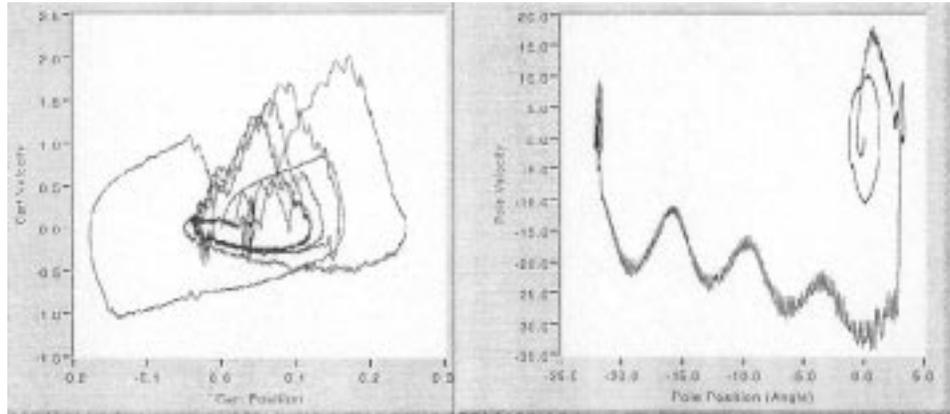
**Fig. 6.** Phase plots for the cart and pole subsystems. These plots illustrate the system recovering from a hard perturbation in pole velocity.
