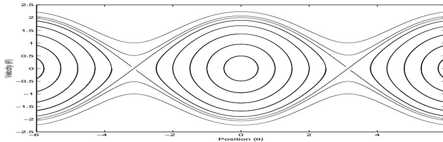
**Fig. 2.** The  $(\theta, \dot{\theta})$  phase portrait of the undamped pendulum. The **Balance** region is an ellipse around the saddle point at  $(\pi, 0)$ . The **Pump** region is contained within the separatrices, and the **Spin** region is outside the separatrices.
