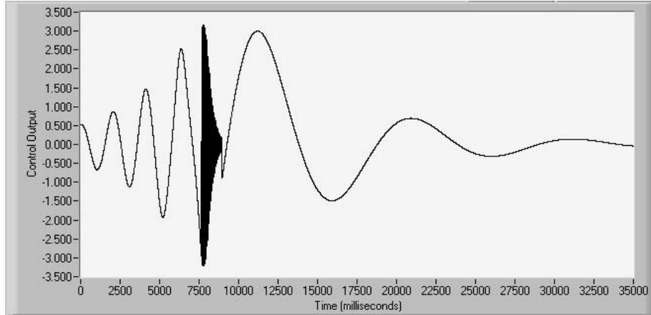
**Fig. 4.** The control action  $u(t)$  shows chattering along the sliding mode.
